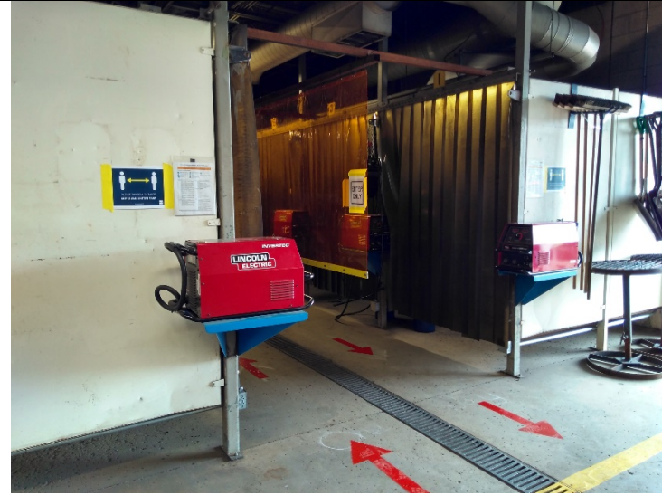
Welding Aisle - Dividing curtain separating students accessing individual areas and path of travel marked on floor at 2m intervals
