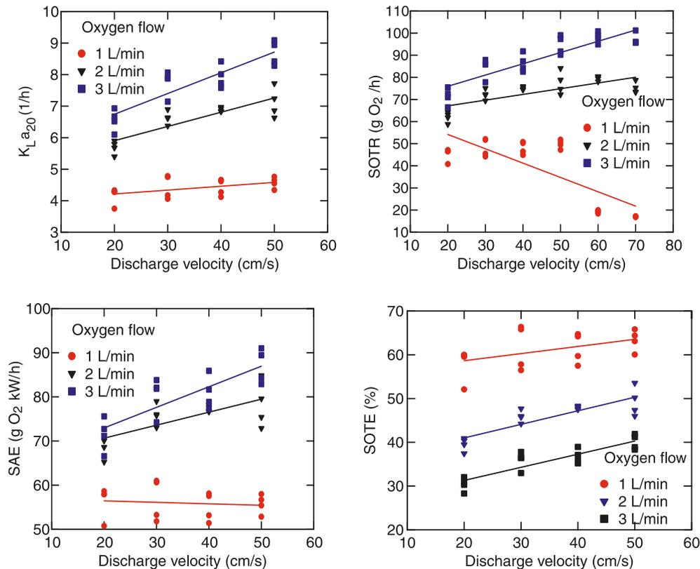
over the range of discharge velocities of 20 to 50 cm·s<sup>-1</sup> (Ashley 2002). However, when operated at combined oxygen flow rates < 2 L·min<sup>-1</sup> and velocities > 50 cm·s<sup>-1</sup>, SOTE decreased abruptly, indicating a collapse of the high oxygen transfer efficiencies normally associated with Speece Cone aerators.
