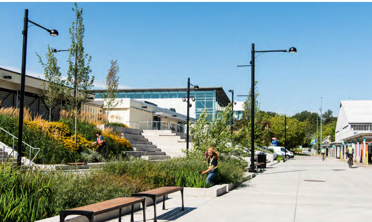
Rain gardens along the Goard Way pedestrian mall provide bio-filtration of water run-off into local waterways, including Guichon Creek.
