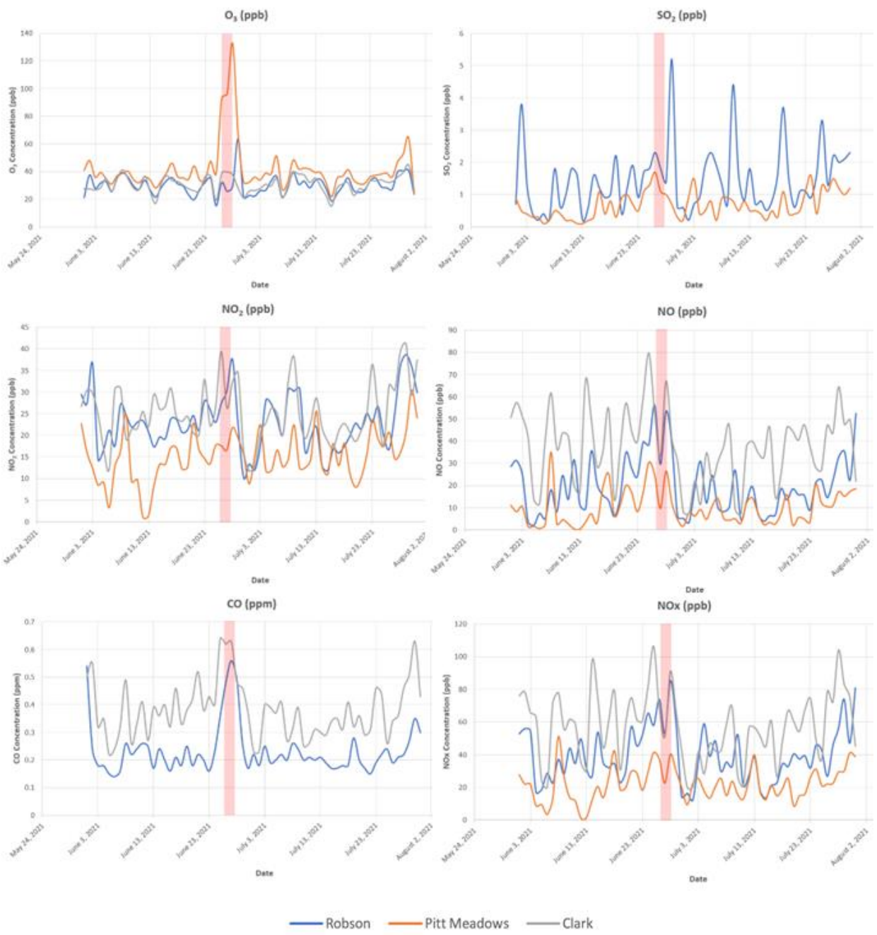
Figure 8. Air Quality Data for June – July 2021. Collected from Robson, Clark, and Pitt Meadows stations' database. Red Highlight Indicates the Defined 2021 Vancouver Heatwave Period (June 26 – June 28).
