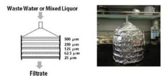
Figure 6. Covered stacked sieve sampling device (reproduced from Lv et al., 2019)
