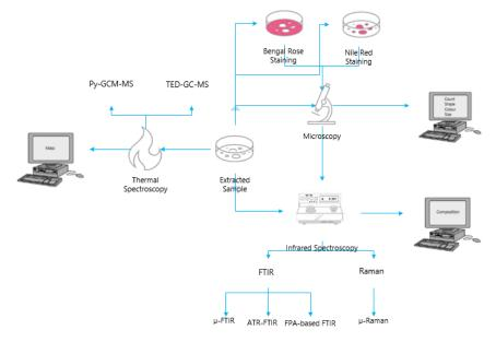
Figure 10. Microplastic in Wastewater Sample Analysis Methods Flowchart (adapted from Bayo et al., 2021)
