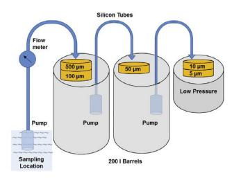
Figure 7. High Volume Automatic Grab Sampling Apparatus (reproduced from Bannick et al., 2019)
