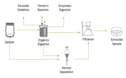
Figure 8. Microplastic in Wastewater Sample Processing Methods Flowchart (adapted from Bayo et al., 2021, and Ben-David et al., 2021)
