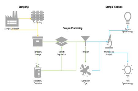
Figure 3. Flow Diagram for Common Microplastic in Wastewater Testing Methods
