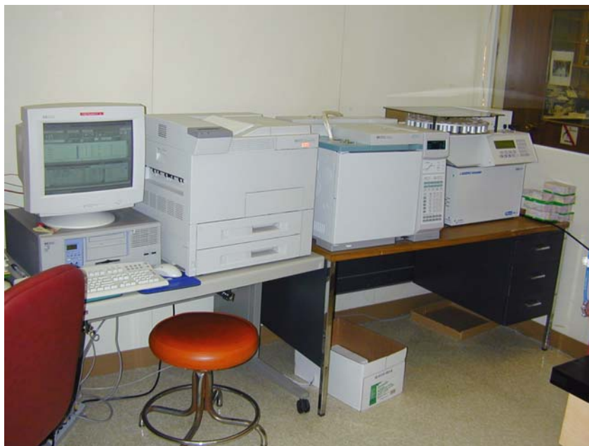
A Headspace Gas Chromatograph used for alcohol analyses
