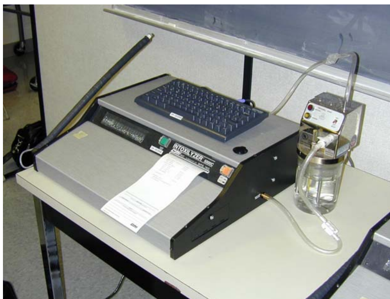
An Intoxilyzer 5000C – one of the approved instruments used in Canada for breath alcohol testing
