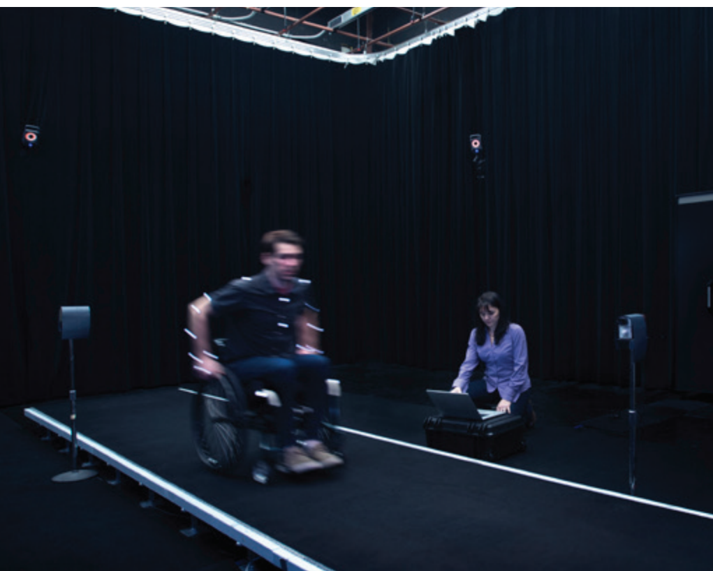
The Motion Capture Lab is a state-of-the-art 3D motion analysis system that records and studies detailed movements of man or animal including joint angles and ground reaction forces in addition to capturing physiological parameters such as body temperature, muscle movement, heart rate, and oxygen uptake
