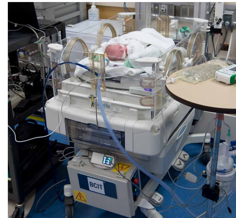
BCIT MAKE+ researchers created a clinical-trial-ready prototype device that simulates skin-to-skin contact for babies who are too fragile to be held by their mothers.
