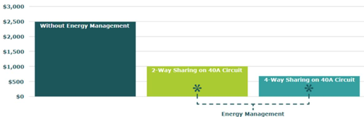
Figure 4: Comparison of cost per energized parking stall of EV charging infrastructure in new construction with various energy management strategies – City of Kelowna. Source: AES Engineering 2019
