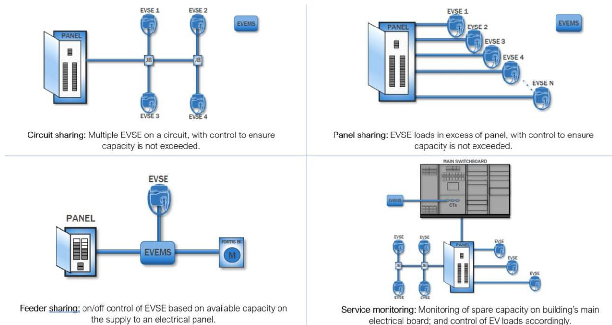
Figure 3: Electric configurations enabled by EVEMS. Source: AES Engineering.
