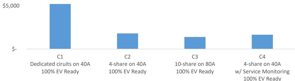
Figure 5: Comparison of cost per energized parking stall of EV charging infrastructure for new and existing developments. Source: AES Engineering October 2021
