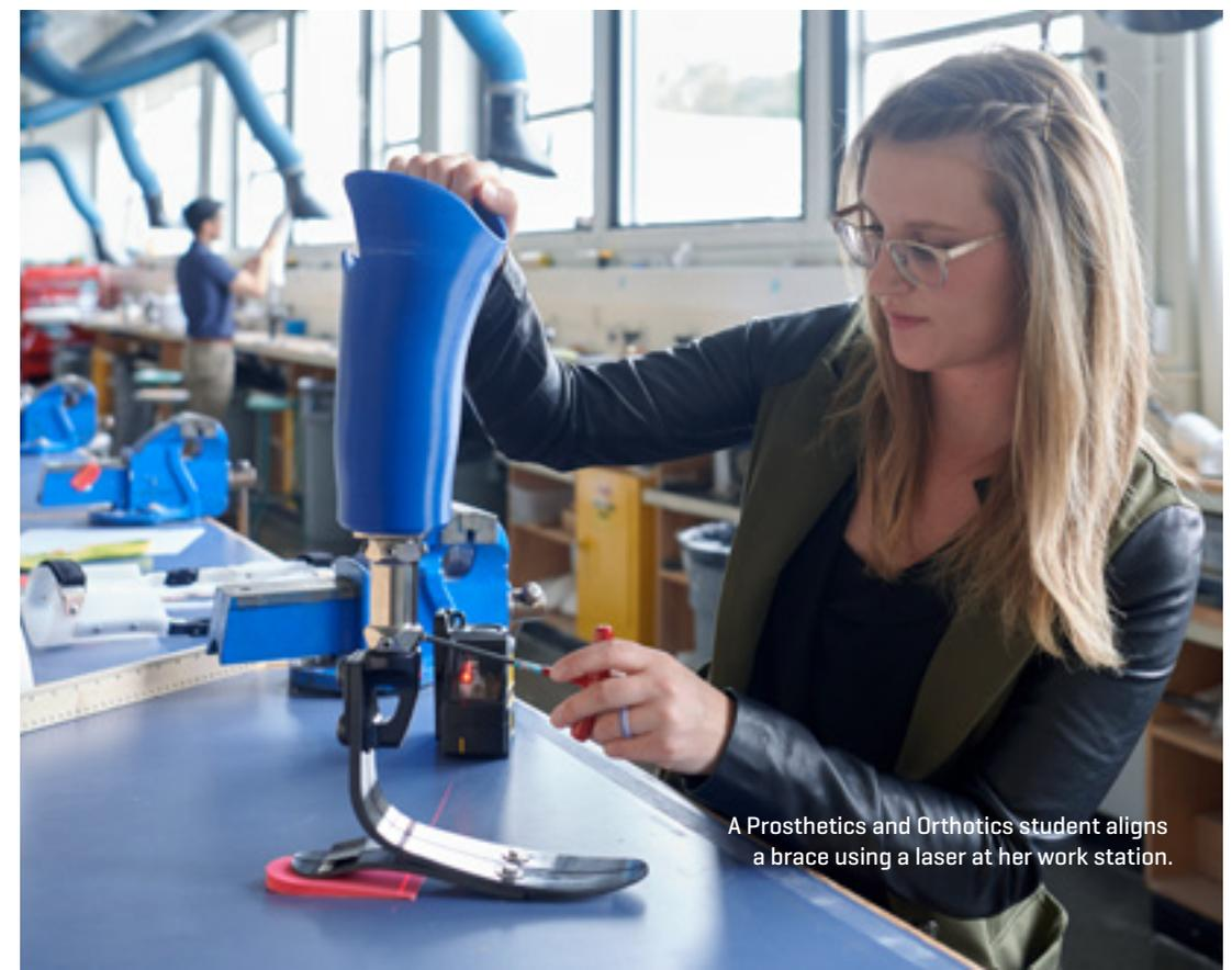
A Prosthetics and Orthotics student aligns a brace using a laser at her work station.
